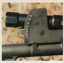
The MGL Mark I is equipped with an Armson OEG collimating-type sight which provides a single vertical red bar. It requires binocular vision on the part of the operator, who aims with both eyes open and sees the aiming bar superimposed on the target
